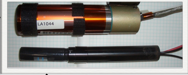
2 types PMT φ34mm, φ15mm
