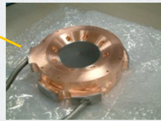
Graphite target with water cooling
