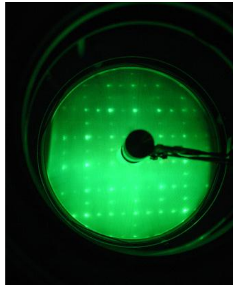
Figure 2.4: A LEED pattern for Si{111}7x7, at 100 eV. The dark object in the middle of the screen is the sample holder.
