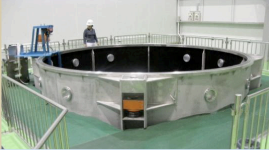
Stainless Steel Vessel (SSV) in assembly pit
