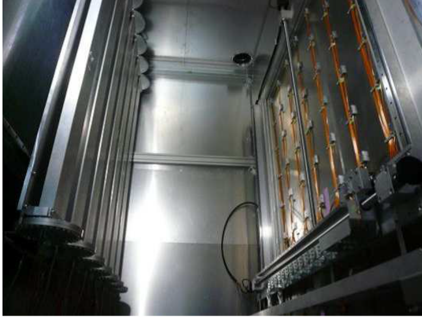
Figure 3.2: Photograph of the silicon PIN photodiodes (right) and the ionization chambers (left) in the support enclosure. The beam enters from the right side. Figure is taken from [88].
