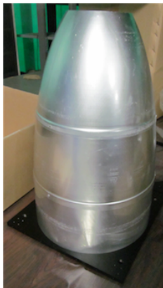
Figure E.3: Photograph of a Winston cone used in BHPV.
