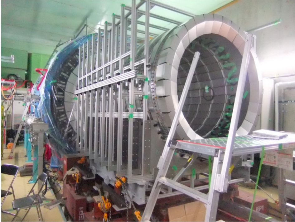
Figure 2.20: Photograph of the IB (forward) just before its insertion to MB (backward). The figures are quoted from Ref. [47].
