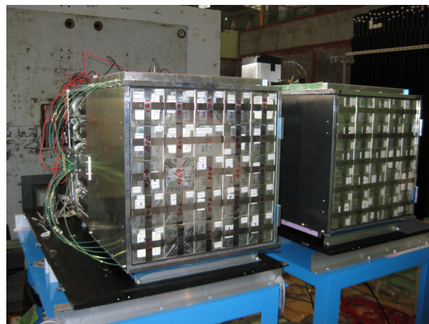
Figure 4.5: Photo of the CsI calorimeter.
