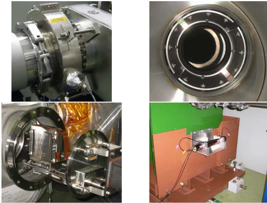
Figure 2.4.: Photograph of the proton-beam monitors. Upper-left: CT (side view). Upper right: ESM (inside view). Lower left: SSEM (being installed in the beam-line). Lower right: BLM (installed beside a normal conducting magnet). These photographs are taken from [12]
