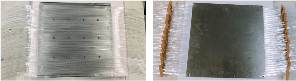
Figure B.1: Construction of the tracking layers made of scintillating fibers. Scintillating fibers glued on the grooved aluminum plates (left) and tagged fibers before inserting fiber cookies (right).
