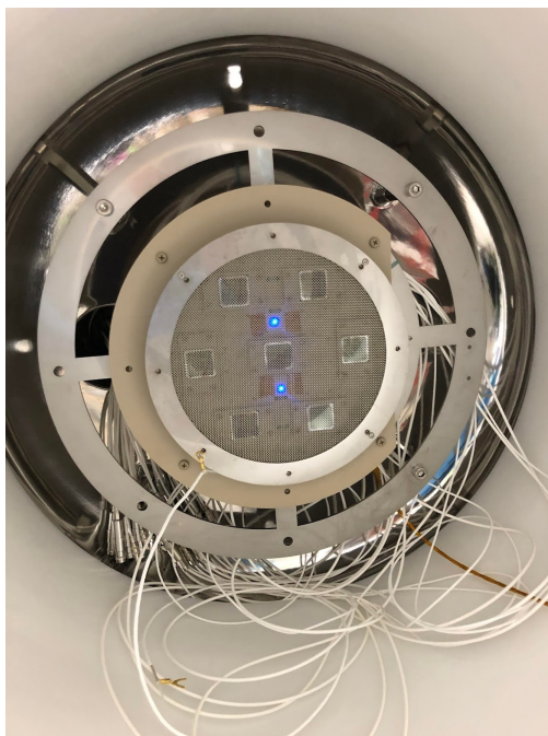
Figure 6.7: LEDs installed in the 180L detector. The LED light is diffused by 0.13 mm-thick PTFE sheets mounted in front of the LEDs.
