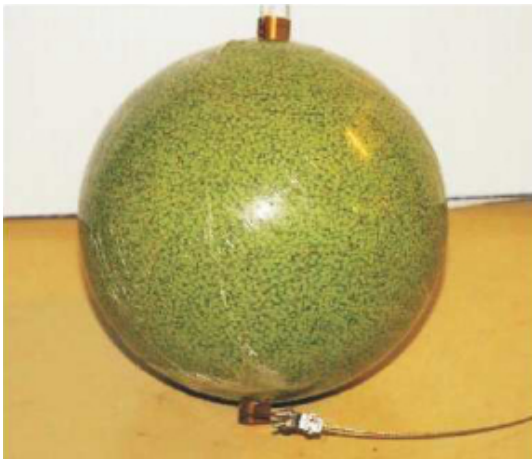
Figure C.10: The nickel ball is a \gamma -ray source [82]. The ball is made of 6.5 kg of NiO and 3.5 kg of polyethylene. The Cf source is inserted into the center of the ball and hold there by a brass rod.
