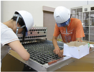
Figure A.17: Connection of the cables with MPPCs on the top readout surface.
