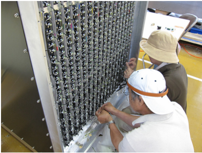
Figure A.13: Attachment of the MPPCs.
