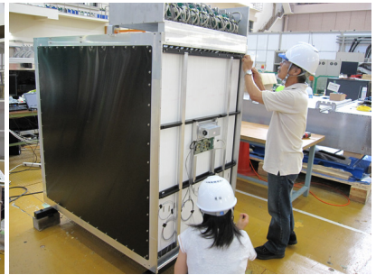
Figure A.18: Attachment of the veto planes.
