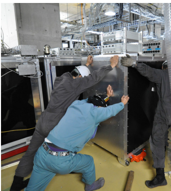
Figure A.21: Photographs of the installation work of the Proton Module (left) and the cables between the Proton Module and the back-end board (center, right).
