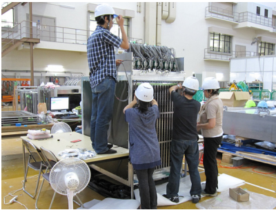
Figure A.16: Connection of the cables with MPPCs on the side readout surface.
