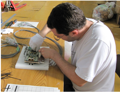
Figure A.14: Attachment of cables to TFBs.
