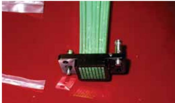
Figure 5.12: The picture of the alignment fixture “cookie”.
