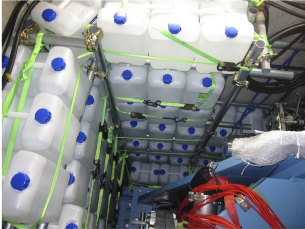
Figure 6.11: Water tanks for the shield. The white tanks with a blue cap are the water tanks. The KOTO detector locates in down-right side of this figure and the primary beam line locates the upside of this figure.
