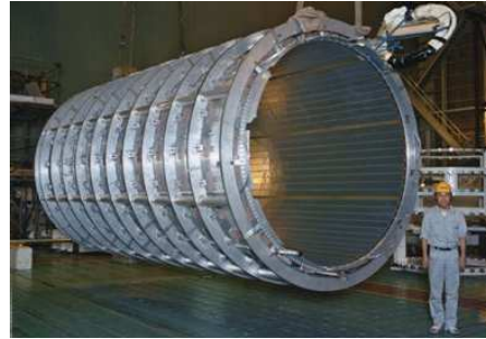
Figure 3.4: Bare central solenoid after completion of the coil winding in the factory.[19]
