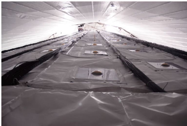
Figure 2.3: A photo looking up from the bottom of the OD. An 8-inch PMT is attached to the wall on the inner tank side, and the outer tank is covered with a white Tyvek sheet.[67]
