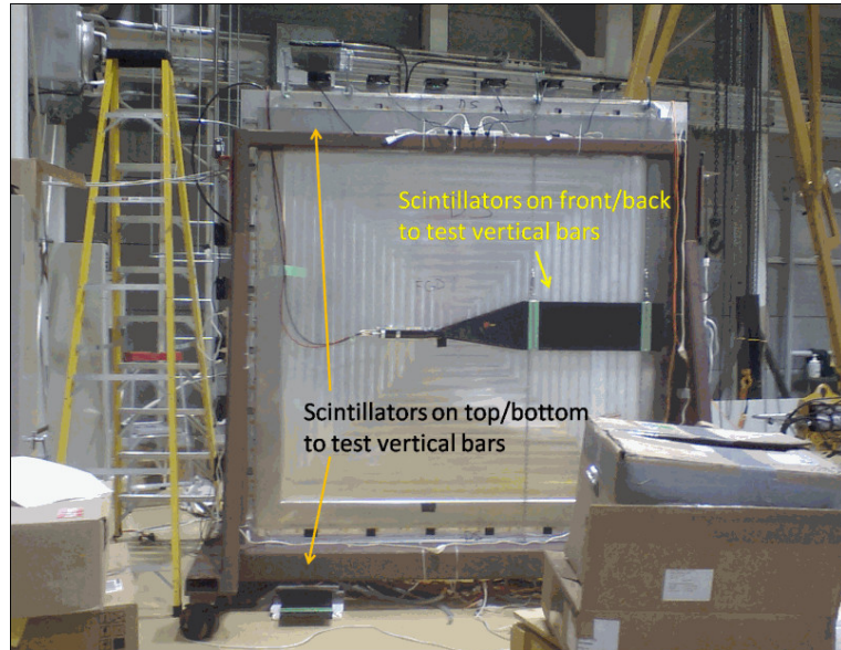
Figure 4.8: FGD1 from down stream side. We hanged 2 \times 2 scintillators on the front/back side of the FGD when we tested the vertical bars, and placed at the top/bottom of the FGD when we tested the horizontal bars.
