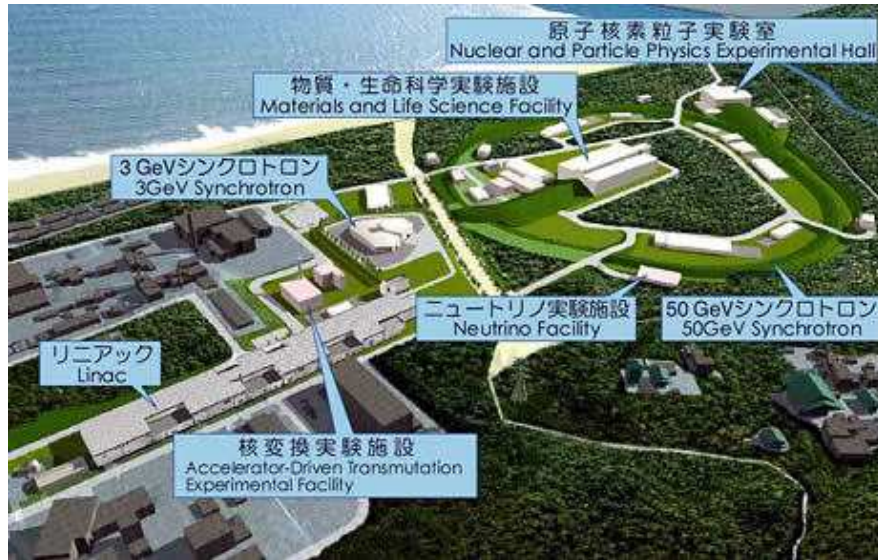
Figure 2.1: Overview of the J-PARC (Japan Proton Accelerator Research Complex) facility. J-PARC consists of the 400 MeV linear accelerator, the 3 GeV proton synchrotron, and the 50 GeV proton synchrotron. It aims to pursue a frontier of science in particle physics, nuclear physics, material physics, life science and nuclear technology.
