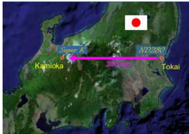
Figure 2.2: Overview of the T2K experiment. An artificial neutrino beam generated in the J-PARC 50 GeV proton synchrotron in Tokai is shot toward the Super-Kamiokande which is 295 km away from Tokai.
