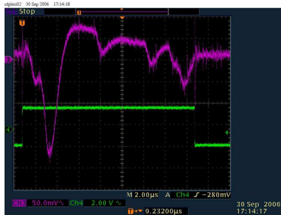
Figure F.7: Output of MPPC through the shaper-amplifier of VA without external light. A pink line shows the MPPC signal and a green line shows “hold_b”. We can see many pileups of the MPPC noise.
